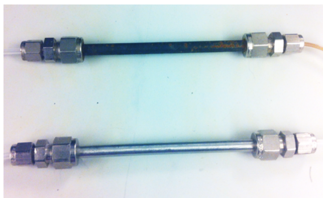
Figure S2. Tube reactors after \text{CaCO}_3 coating treatment. The upper reactor is made of mild steel and the bottom one is made of stainless steel.
